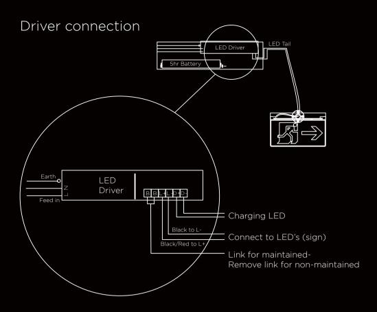
Charging LED - to be wired into LED Driver D+ & D-LED Wire - to be wired into the LED Driver L+ & L-Earth Wire - attach to the LED Driver fixing screw 240v supply to be wired to LED Driver L & N
